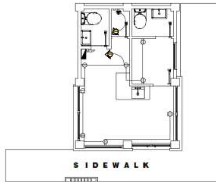
GUARD HOUSE POWER LAYOUT SCALE: 1:100 M
